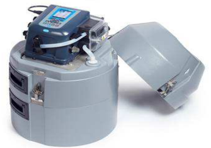
Auto Sampler – Portable Automated Water Sampler with 10 litre capacity for streams, surface and ground water
